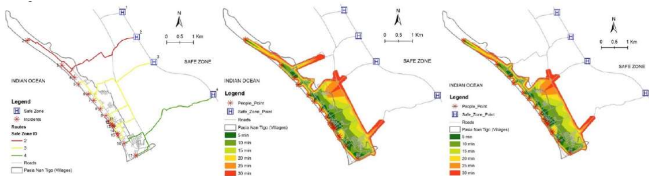
Figure 5. (a) Closest Facility analysis, (b) Service area 30 min from beach towards safe zone, (c) Service area 30 min without Bridge 1
